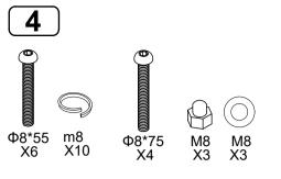
Carefully lower and align frame left hand side part B onto assembled frame with one person supporting the frame ,the other person can add the screws with washers as shown.hand tighten .slowly tip assembled frame to upright position, and check all screws are sufficiently tightened.
