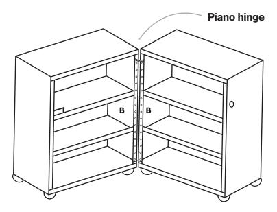
1. Position units as shown. Fit Piano hinge to ends B using (30) 5/8 x 4 screws.
