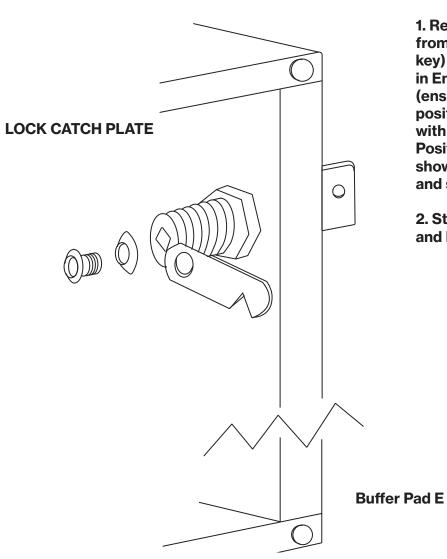
1. Remove screw and washer from key barrel (do not remove key) Insert barrel through hole in End C and secure with nut (ensure key is in the vertical position before tightening nut with spanner).
