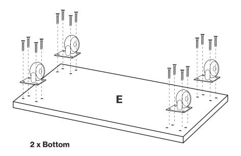
1. Secure 4 Castors to bottom using 1/2 x 8 screws into 'POP' marks (lockable castor to front or rear).
