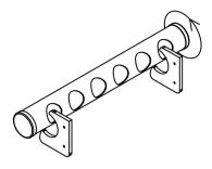
Put the opening of the plant planting pipe on the PE board, and then rotate it into the slot.
