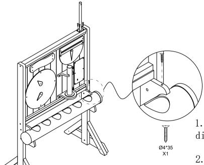
1. The measuring cylinder should directly stick into the slot  $\!\!\!_{\circ}$
