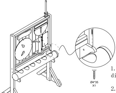
1. The measuring cylinder should directly stick into the slot.
