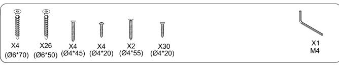
DO NOT FULLY **TIGHTEN SCREWS** UNTIL ALL SCREWS HAVE BEEN LOOSELY POSITIONED.
