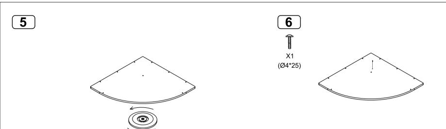
Embed the lamp into the base ,rotate and fix it
